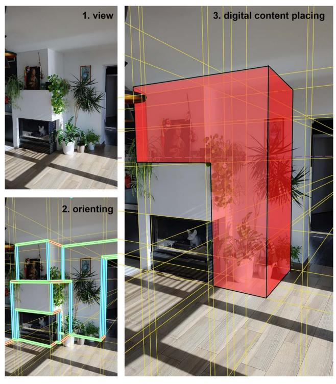
Figure 2: Augmented reality in use - 1) view capture; 2) description of coordinates and orientation; and 3) placing oriented digital 3D content - endless loop for real time effect (Author's materials).
