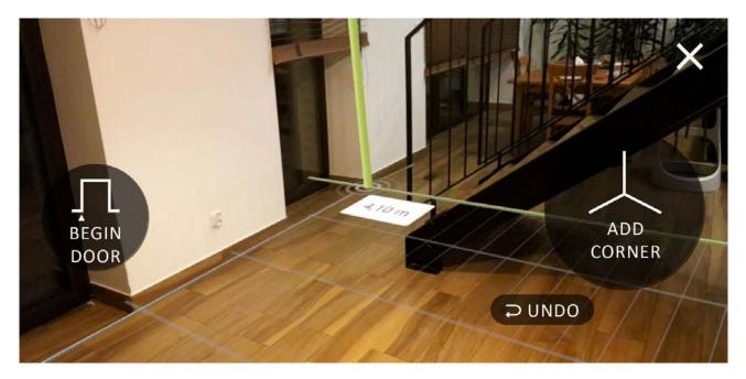
Figure 3: Example of the *magicplan* app screen. After calibration a starting point is set on one corner of a room; then real time measurements are available. Locking the positions of all edges will lead to a compact plan of the room (Author's material).
